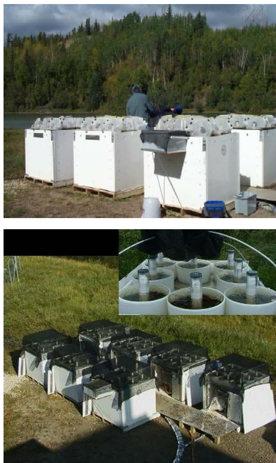
Figure 9-2: A) Small microcosm system with streams situated on tables over mixing reservoirs used in the Thompson River, British Columbia. B) Modular mesocosm system with streams situated on tables over mixing reservoirs used in the Little River, New Brunswick; Junction Creek, Ontario; the Wabigoon River, Ontario; and Key Lake, Saskatchewan.
